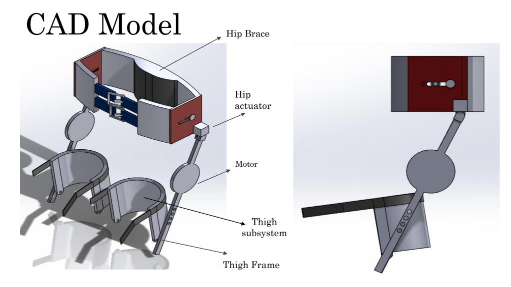
Figure 2: isometric view of CAD design
